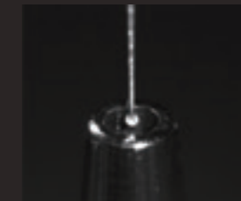
Measurement using MPP-NANO stylus
